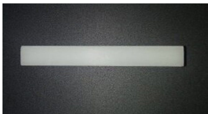
Figure 1. Polyethylene block prepared in the dimensions 4x10x80 mm
