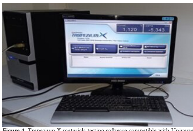
Figure 4. Trapezium X materials testing software compatible with Universal testing machine
